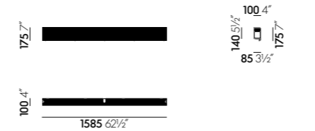
Dancing Wall 2, electrification channel
